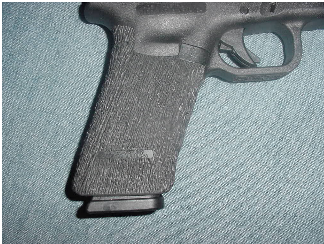
Close-up of Bowie Tactical Glock grip reduction
