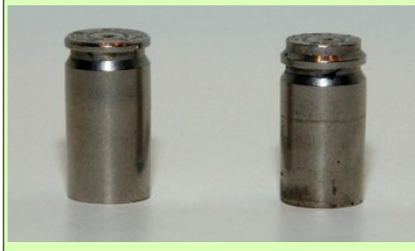
The photo at left shows an improperly extruded case (R) compared to a properly formed case of the same ammo (L). The bad round fed into the gun and fired properly, but because the extractor groove and rim are in the wrong place there was no way for the extractor to grab the case and it had to be punched out from the muzzle. Obviously, that's a problem you cannot expediently
