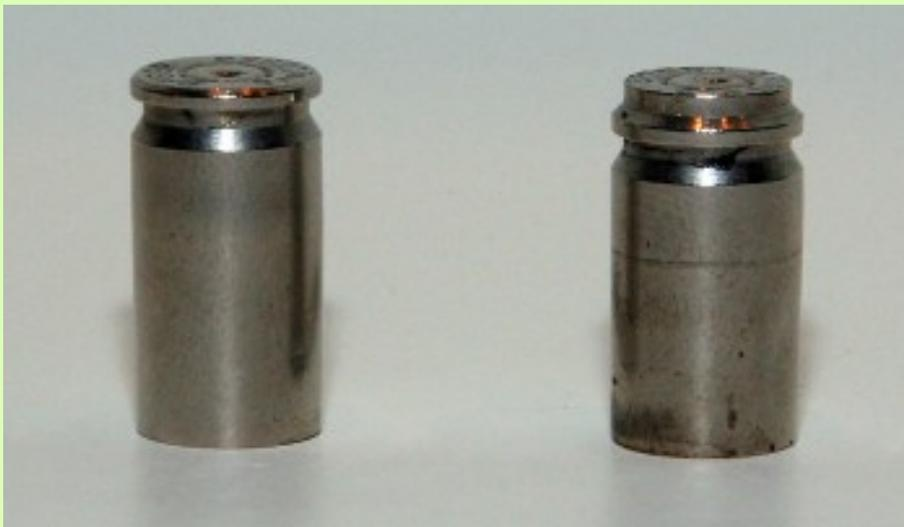
The photo at left shows an improperly extruded case (R) compared to a properly formed case of the same ammo (L). The bad round fed into the gun and fired properly, but because the extractor groove and rim are in the wrong place there was no way for the extractor to grab the case and it had to be punched out from the muzzle. Obviously, that's a problem you cannot expediently
